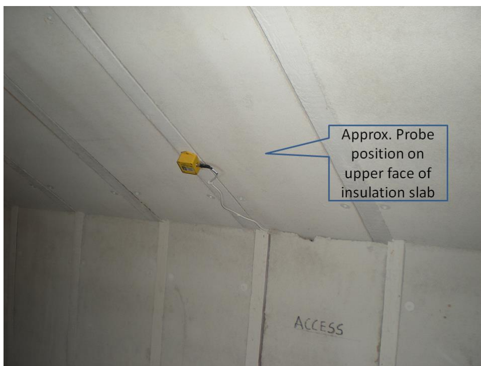
Figure 4: Location of temperature/RH probe above insulation slab in attic.
