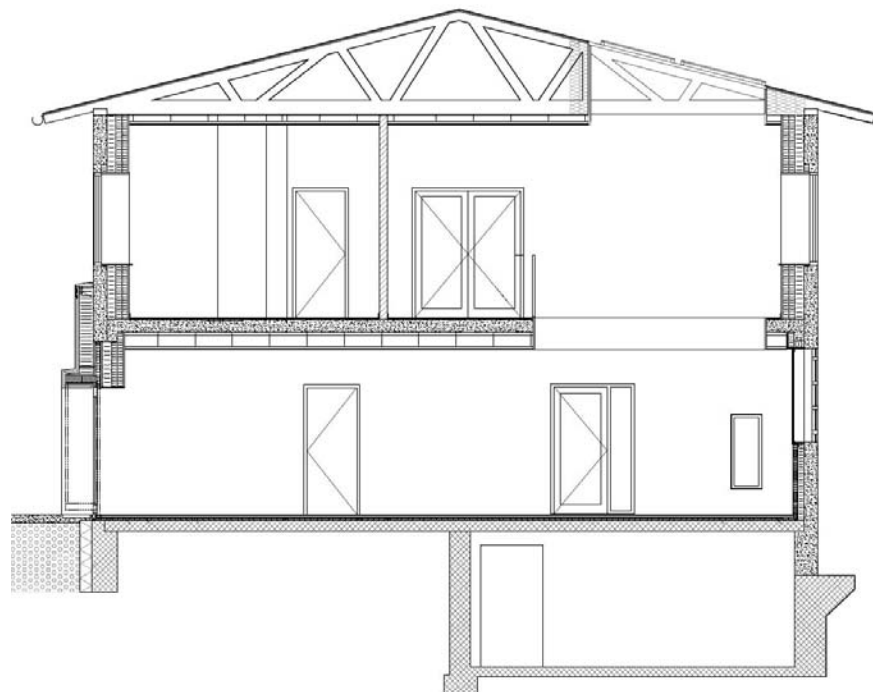
Cross section of the energy-renovated building.
