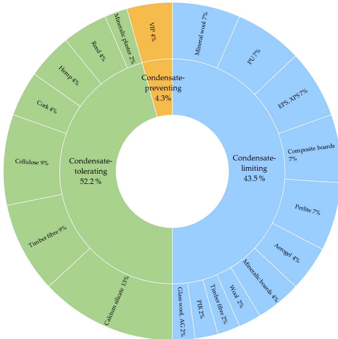
Figure 18: Sunburst diagram showing the share of different insulation systems in published case studies grouped by their insulation system class: condensate-tolerating (green), condensate-limiting (blue) and condensate-preventing (orange).
