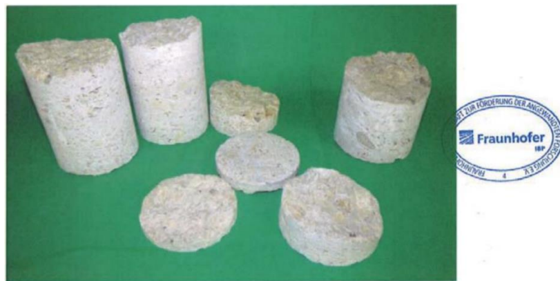
Figure 61: Samples from Brüttelen quarry of shell limestone probably used for the construction of the monitored building. Picture taken by IBP.
