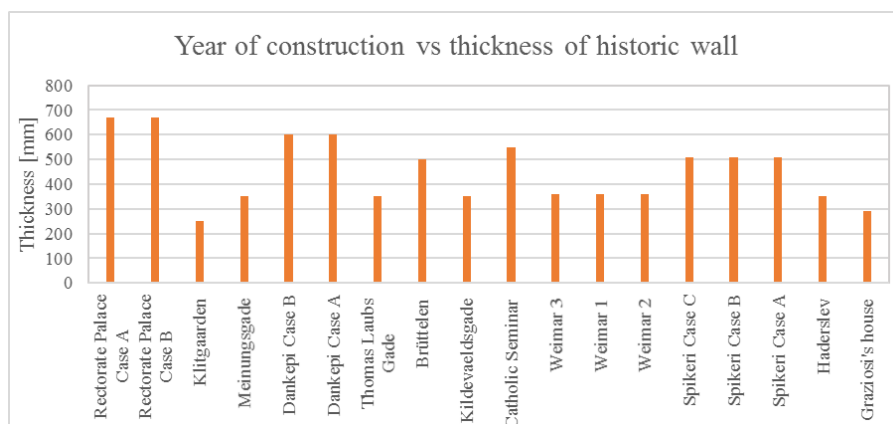
Figure 13: Wall thickness (original historic construction) of the RIBuild case study buildings ranked by their year of construction (starting with the oldest building from 1866).
