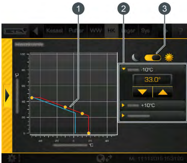
Fig. 5-65: Heating curve settings
