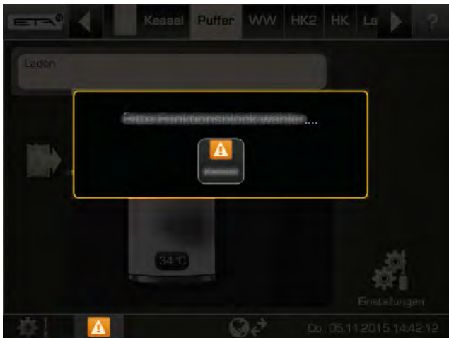
Fig. 5-10: Display of the function blocks in which the error occurred
